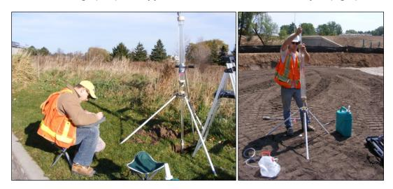
Figure 5.3 - Infiltration Testing Conducted During IMAX Parking Lot Reconstruction Project – Mississauga (left) and Upper Middle Road Bioretention Project (right)
